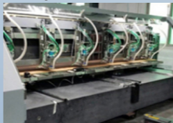
PCB钻孔机 PCB drilling machine
